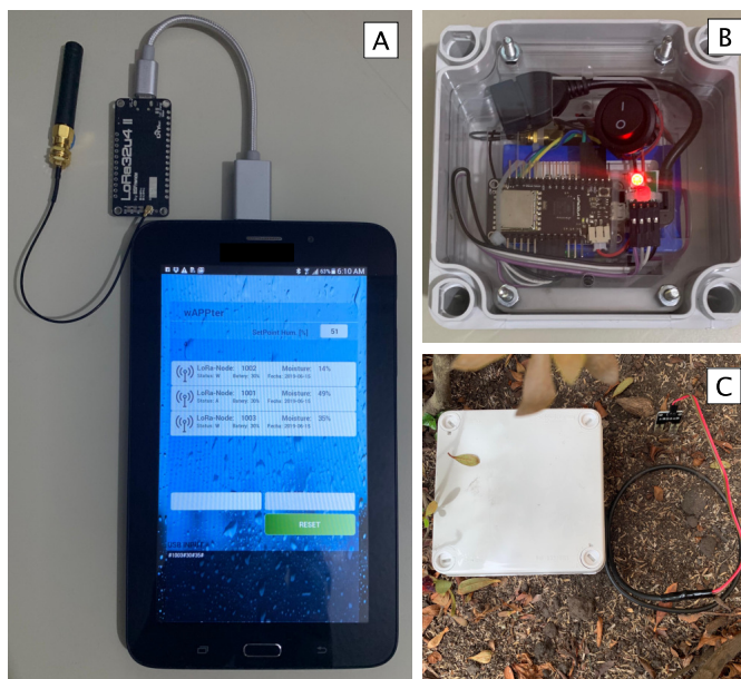
Fig. 3. Front Layer components. (A) Lora-Gateway, (B) Lora-Node, (C) Lora-Node on a cloudy day at 30°C
