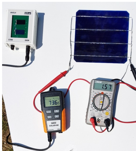
Fig. 11 Irradiances and short circuit current measured on field test.
