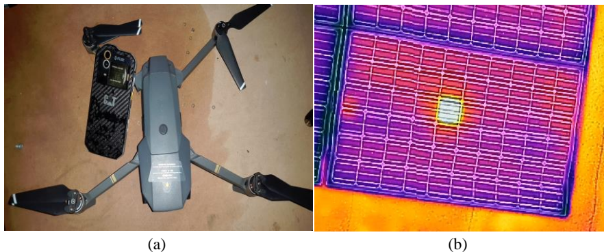
Fig. 14. Solar panel thermography with drone (a) Cat s60 thermal camera and DJI Mavic Pro drone (b) captured the image.
