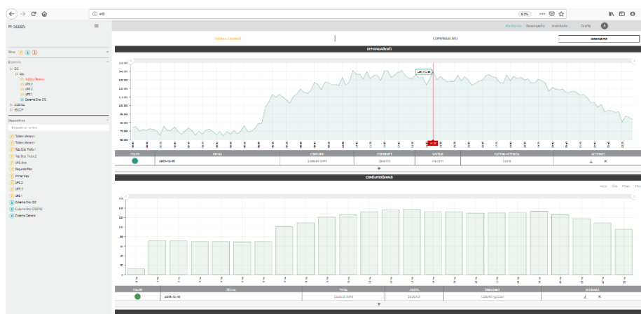
Fig. 4. Electricity consumption as registered in the SEEDS platform at CIC on 2018-12-18.
