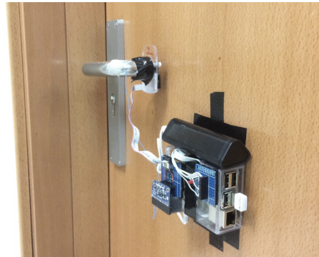
Fig. 3. Snapshot showing the acquisition platform affixed to a door and to the lever doorknob
