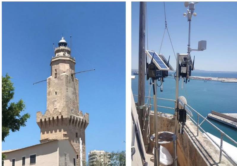
Fig. 5. Sensor Platforms installed in Portopí Lighthouse
