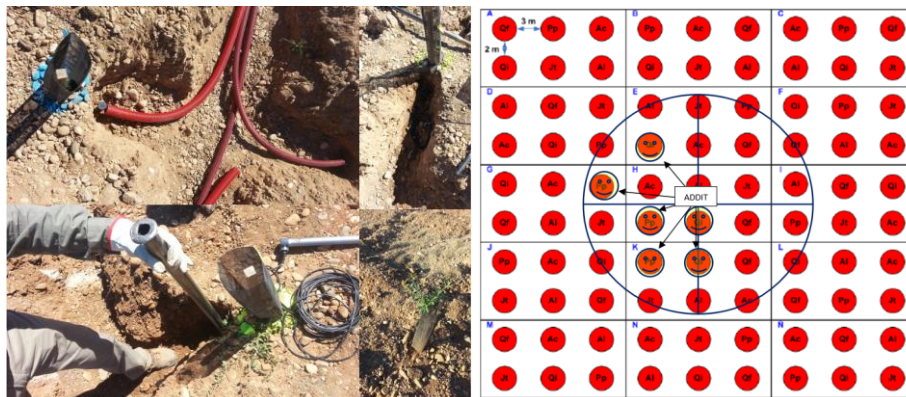
Fig. 2. Installation of the soil sensors (left) and diagram of the data capturing system for each plot (right).
