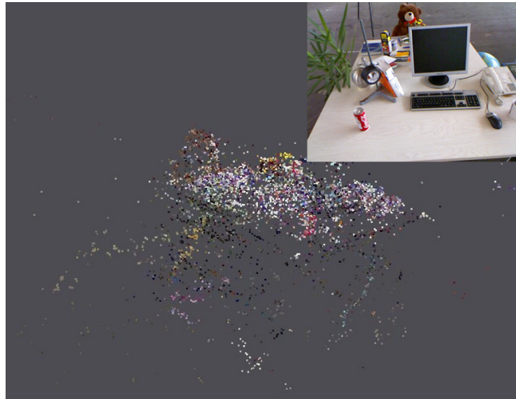
Fig. 1. The point cloud of a desktop generated by SLAM methods. In addition, this point cloud allows the system to determine the camera position on future trajectories.
